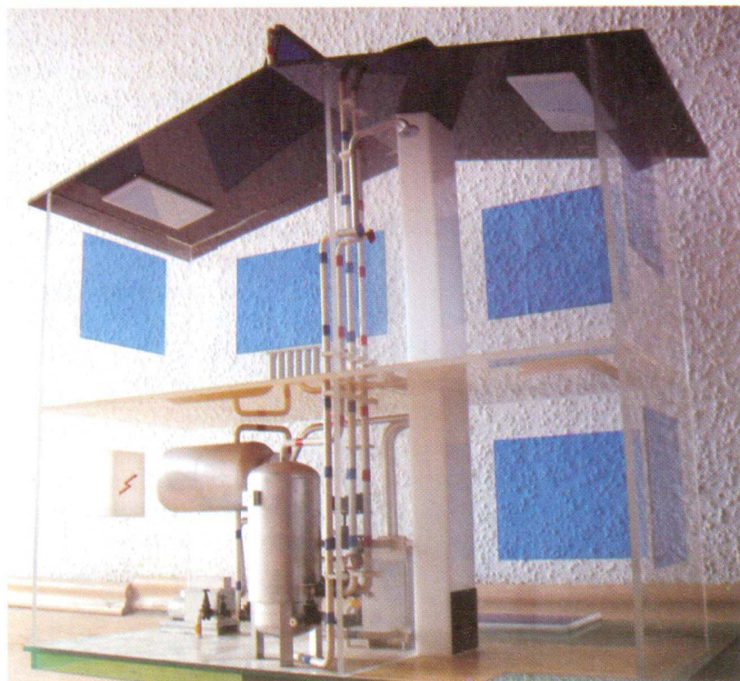
Fig. 7. Model of the author's home in Szczecin which in 1993 was equipped with gas-fired CHP plant, hot water and electric radiant heating, solar panels, 900 litre thermal buffer coupled to the heat pump, fireplace with an air jacket and hot air distribution to three rooms.
