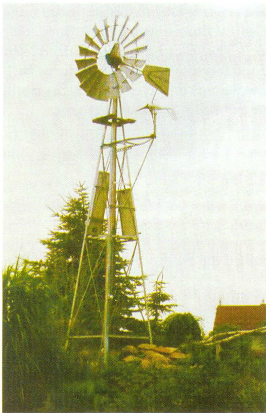
Fig. 1. Windmill-driven pump operating in Łędzin near the Polish seaside.
